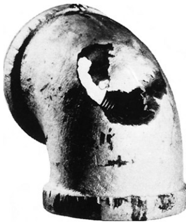
Figure 6.10 Impingement failure of an elbow that was part of a steam condensate line.
